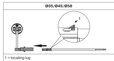
Plug the **dead** connecting cable into the angled plug until the locating lug clicks into place in the angled plug. If necessary, use a suitable flathead screwdriver to assist with insertion. Set the screwdriver into one of the two grooves on the plug-in connecting cable provided for this purpose.
