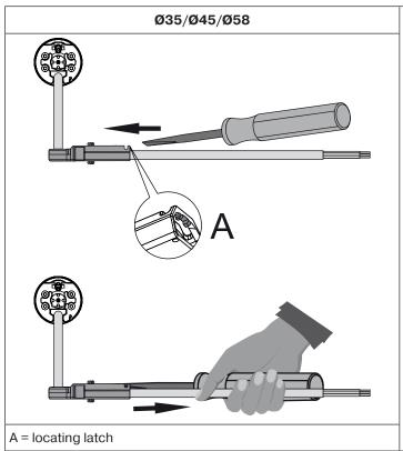
Insert a suitable flathead screwdriver right into the recess of the locating latch, so that the latch releases the locating lug from the plug.
