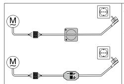
Automatic setting of limit positions is possible, where a stop system is present on both sides, using the rotary switch set (Item no. 4901 001 158 0), a standard rotary switch or the programming unit for drives with electronic limit switching (Item no. 4935 200 011 0). All other functions can only be set via the programming unit.
