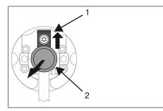
When pushed in, the mounting pin (2) locks automatically. To undo the mounting pin (2), push the tab washer (1) upwards and pull out the mounting pin (2).
